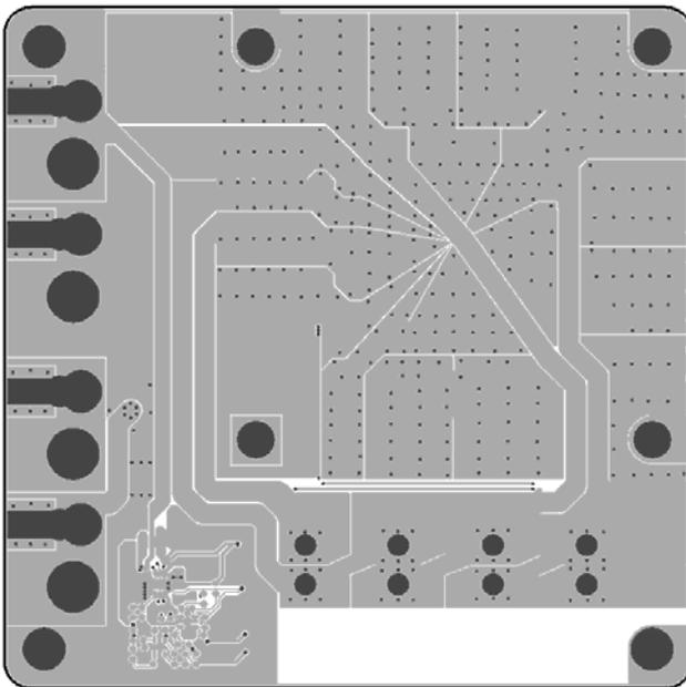
Figure 4. Top Layers without Top Screen Layer
