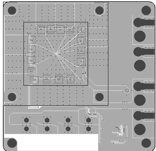
Figure 6. Mirrored Bottom Layers
