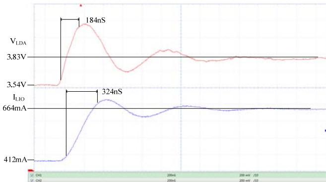
9 Laser Diodes U_1=3.3V , R_D=1.23\Omega
